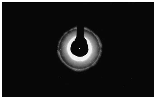
Fig. 6. Same as Fig. 5. Electron diffraction image of palagonite [32].
